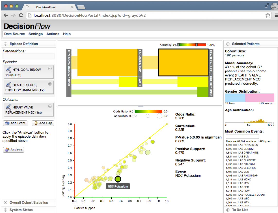
Fig. 3. In this example, a user has used a modified version of DecisionFlow to segment the example population into subgroups based on the appearance of specific features in the data. Predictions for each subgroup have differing levels of prediction accuracy as illustrated by the color-coded bands in the top portion of the visualization. The scatterplot view shows individual features that associate strongly within the subgroup with correct (green) or incorrect (red) predictions and can be used to interactively define additional subgroups. Once a problematic cohort is isolated, users can quickly send the samples to the linked PARAMO platform to begin training a new predictive model that targets the narrower, more focused set of examples.
